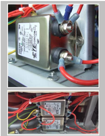
Top: one EMC filter unit (1000W e2s variant) Bottom: two EMC filter units (2000W e2s variant)
